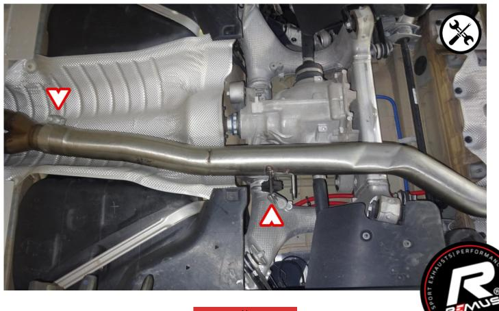
Mount the standard actuator and the standard heat shield with the supplied spring on the left REMUS valve tube. If necessary, slightly spin the actuator, suitable for the spring, so that you can mount the actuator properly!
