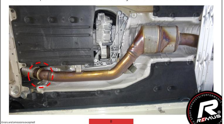
Unhook the rubber hangers, unplug the actuators and remove the standard exhaust system.
