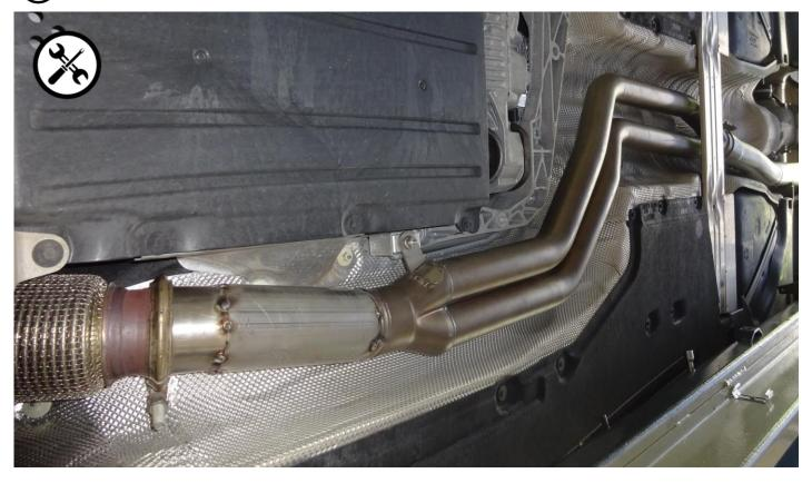
Mount the connection tube onto the front silencer replacement and hang in the rubber support.
