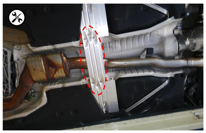
Loose the clamp connection of the standard between catalytic converter and front silencer.
